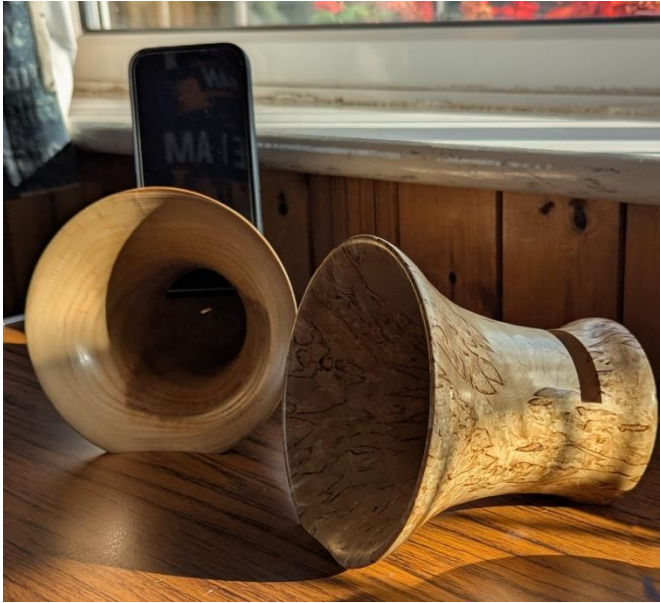
These speaker horns were made by Mike C – used as a phone stand they amplify the sound.
